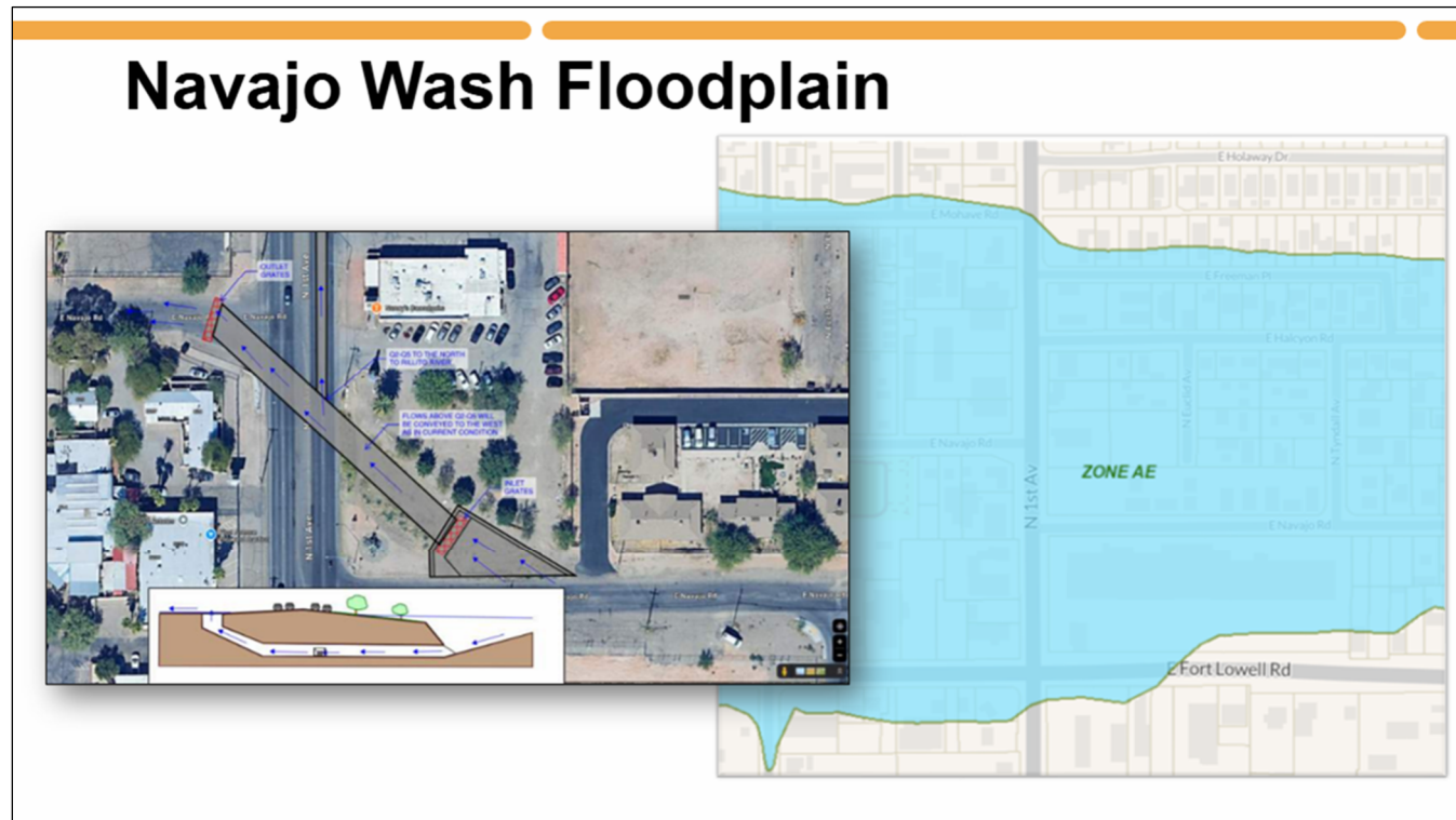
Figure 48 – Conceptual Layout of Proposed Navajo Wash Floodplain Inverted Siphon
